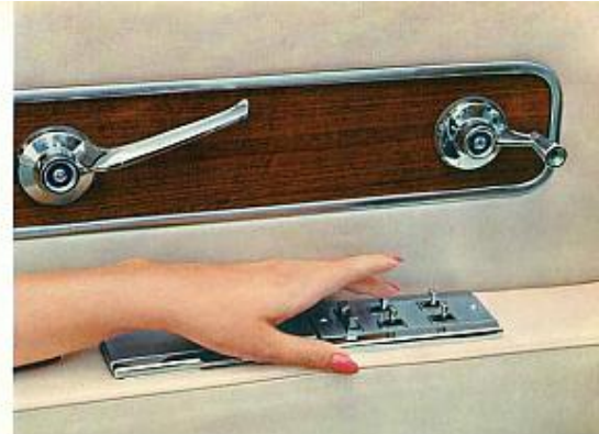
This panel, set into the armrest of the left front door, gives the driver finger-tip control over the power windows built into every Lincoln Continental. Individual control switches at each window permit passengers to raise or lower their windows; the driver can lock out these controls, when desired, by pressing a switch on his control panel. Notice the elegant walnut door paneling.
